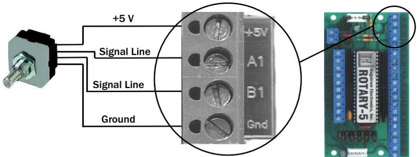
**Mechanical Rotary Encoder Hookup:** To connect a mechanical rotary encoder to the ROTARY-5, use the arrangement shown below. Mechanical devices only require the Ground connection and two signal connections. No power connection is needed for the mechanical rotary encoder.
